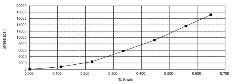
\*Young's modulus is calculated using the secant modulus at each data point per Figure 2 (C) in ASTM D 7012
