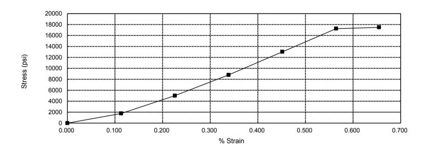
\*Young's modulus is calculated using the secant modulus at each data point per Figure 2 (C) in ASTM D 7012
